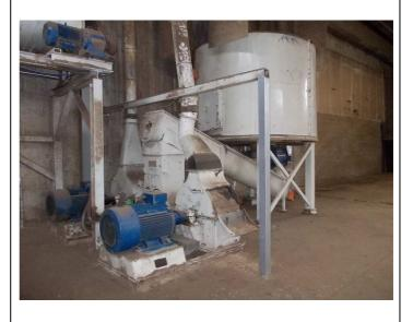
4 - SPIRAL MIXER for fine materials from 5 cubic meters, with the support system.
