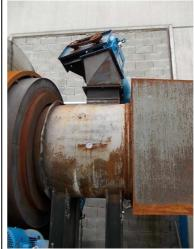
5 - DRYER DRUM 3 steps,mod. ROTAR 250 external drum size 2500 x 9300 mm
