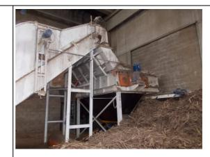
2 - STAR VALVE and screw for dosing and feed hammer mills with discharge hopper complete of magnets. Power installed: kW 4,4
